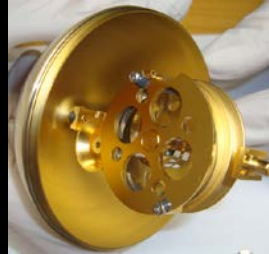
Titanium Nitride probe hemisphere and gold-plated yoyo mechanism
